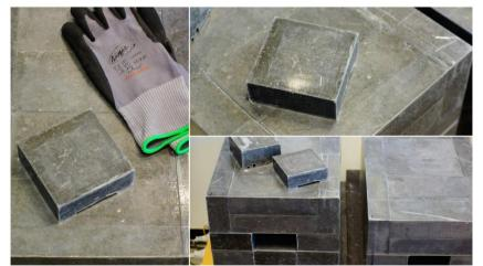
or assemble the shielding according to the instructions supplied by DTU Nutech, and then wrap the entire lead shielding in plastic foil.
