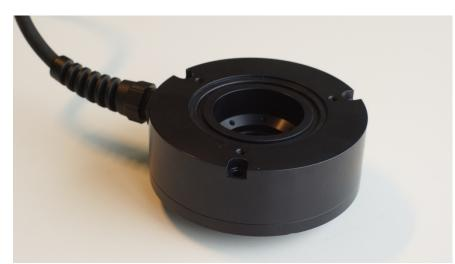
The OSL unit enables flexible and combined BLSL/IRSL/TL measurements in automated sequences. The OSL/IRSL system includes a software controlled power supply to allow illumination power to be varied during a measurement sequence (e.g. for normalisation) or to ramp of the illumination power during an OSL readout to perform linearly modulated OSL (LM-OSL) to investigate trap distributions and OSL decay rate components.
