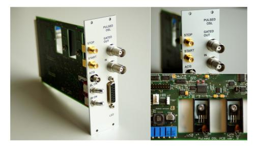
The unit is e.g. suitable for separating quartz from feldspar OSL signals in feldspar contaminated samples.
