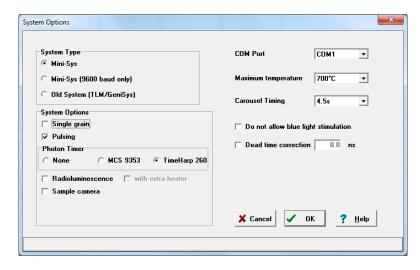
To acquire Photon Timer Data from a Pulsed OSL stimulation you just mark "Enable Photon Timer data acquisition" as show in the POSL dialog in the figure below
