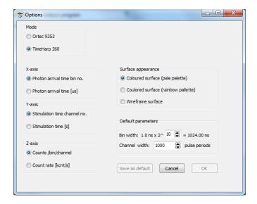
In the *Mode* box you select the board that your Photon Timer attachment is equipped with.
