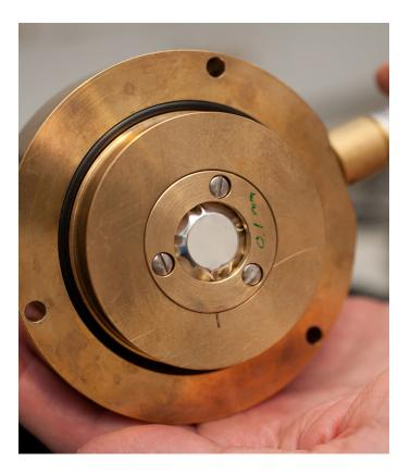
Figure 2.8: The x-ray collimator window.
