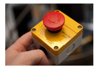
Figure 2.4: The x-ray emergency stop.
