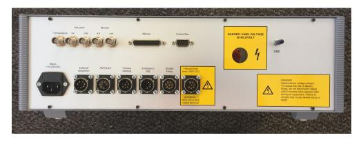
Figure 2.12: Labels on the back of the XHV-1 control unit.
