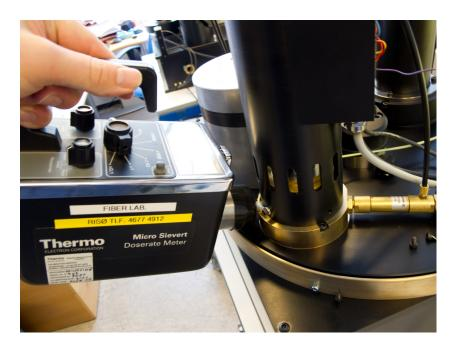
Figure 2.3: The x-ray tube during leakage testing.
