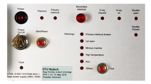
Figure 2.6: Indicators with status information on the front of the XHV-1 control box.
