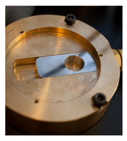
Figure 2.7: The x-ray collimator block with mechanical shutter.
