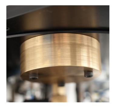
Figure 2.10: The beam stop below the x-ray collimator (shielding removed).
